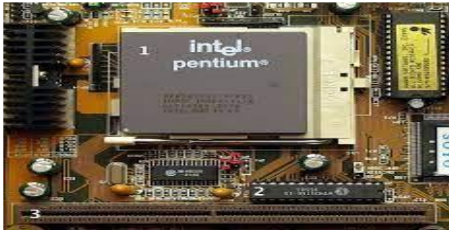
Figure 20 The CPU inside the computer motherboard
